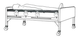
**6:** For mattress overlays and **0.R.** Pad: To adjust for the proper immersion level of each product section, slide your hand between the product surface and the individual's lowest bony prominence. Turn the valve **counter-clockwise** to open, and release air until the area of high risk is within the suggested Inflation Guidelines (see the next page). Turn the valve **clockwise** to close. Repeat Step 6 for the remaining product sections.
